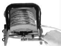
To Test Entire System Hold the contre pin on the probe against the stud on the back of the axle at the same time touch the probe body aginst the screw on the frame. The buzzer will sound if the system is ok. Sensitivity knob should be turned fullly clockwise.
